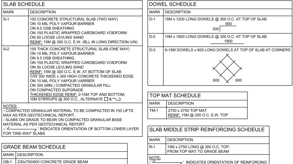
REINF: 2-20M HORIZONTAL BARS TOP AND BOTTOM,
